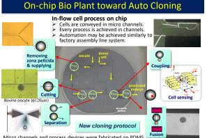
Micro channels and process devices were fabricated on PDMS Fusion chip(Collaboration with Tohoku U., AIST, NLGS, KHI, and Fujihira) AROB, INBOG JRM10, JRM13
